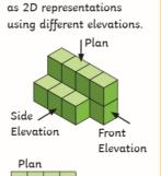
Front Elevation Side Elevation
